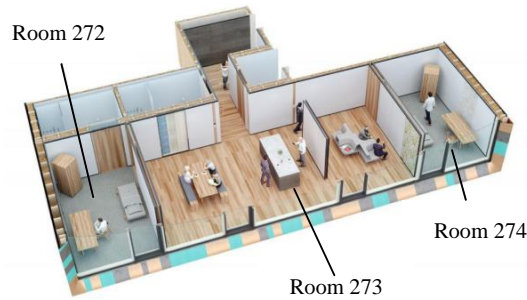
Figure 5.13: Layout of the UMAR unit with the controlled rooms marked. © Werner Sobek.
